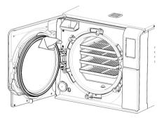
5 Insert the new seal and press first up and down.
