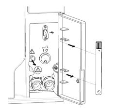
Insert the opening tool into the hole and then turn it counterclockwise until the door is unlocked (proceed slowly until it stops).
